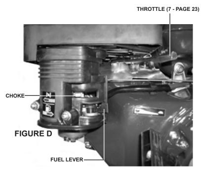
2. To start the Engine, turn the Fuel Lever to its "OPEN" position. Turn the Choke to its "START" position. Then turn the Throttle to the RIGHT to its "SLOW" position. (See Fig. D.) Note: If the Engine is already hot, keep the Choke in the "RUN" position.
